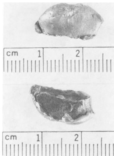
FIG. 2.—Two views of the single distorted pellet that was consistent with 0 buckshot.
